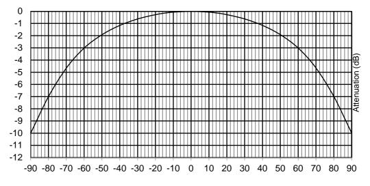
Figure 5: Minimum attenuation of the horizontal antenna pattern
