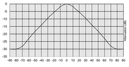
Figure 4: Minimum attenuation of the vertical antenna pattern
