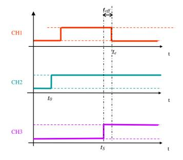
Figure 11: Maximum transmit switch-off time, toff, measurement
