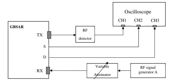
Figure 8: DAA measurement arrangement
