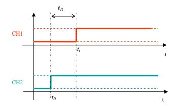
Figure 9: Minimum listen time, t<sub>D</sub>, measurement
