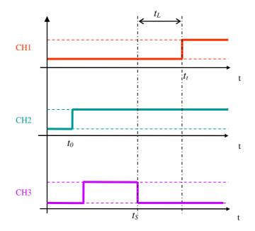
Figure 10: Minimum listen time after detection,  $t_L$ , measurement
