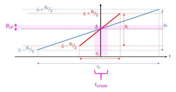
Figure E.2: Crossing time  $\ensuremath{t_{cross}}$  between interfering signals
