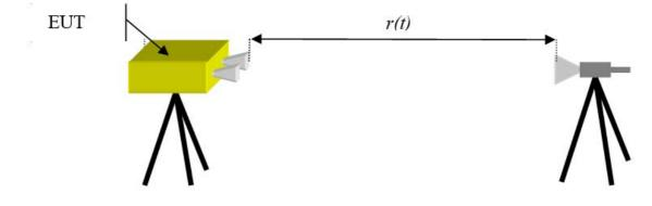
Figure 7: Setup for RBS measurement
