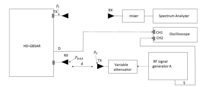
Figure 12: DAA measurement arrangement
